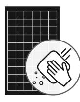
It is recommended that installation, changing and maintenance of the modules is implemented by an authorised service technician. Regular maintenance and cleaning of the modules is highly recommended for them to function well and properly. At regular visual inspection carefully check the condition of glass and frames, possible corrosion, the presence of moisture under the glass, overheating or colour changes at ribbon joints, condition of connectors and electrical cables.
