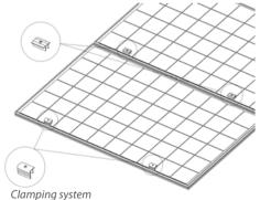
The modules should be mounted basically at the 4 quarter points by the means shown in the picture. Metals used in locations that are exposed to moisture shall not be employed alone or in combinations that could result in deterioration or corrosion. The maximum torque of the clamps should be applied according to the clamping system design request. Please be alert that overtightening might cause module damage.
