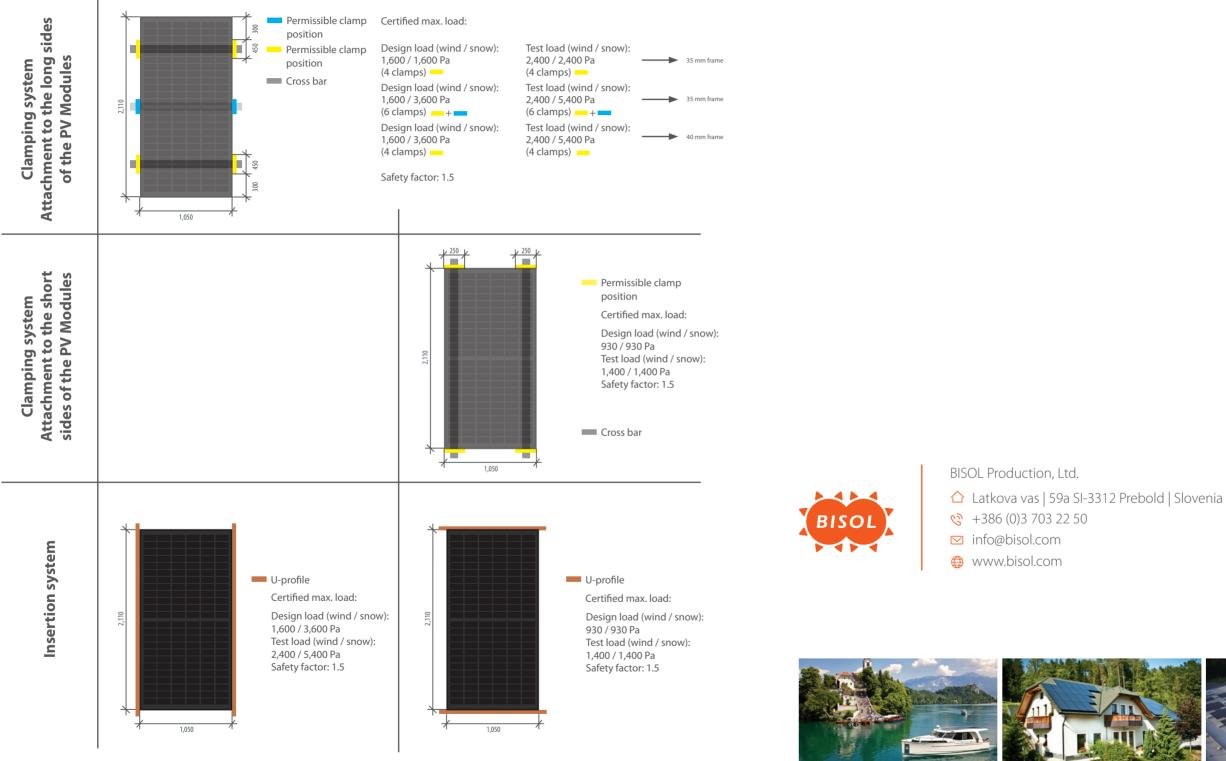
All the tests are made according to the IEC 61215:2016.
