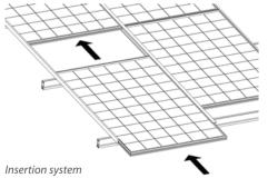
The module may be mounted on the support by using an appropriate insertion system with or without additional clamps. The insertion system may fasten the long or the short side of the module frame.
