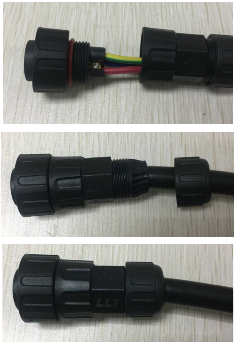
Fig.13. Reassemble the AC connector
